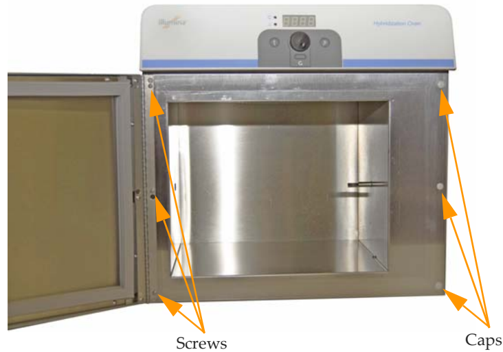
Figure 4 Reversing the Illumina Hybridization Oven Door
