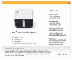
2 Confirm that the **Instrument ID** number on the screen is the same as the instrument serial number on the back of the Eco instrument.
