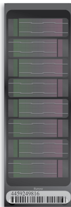
Figure 1: Infinium Global Diversity Array with Enhanced PGx-8 BeadChip—Built on the trusted eight-sample Infinium LCG assay platform.
