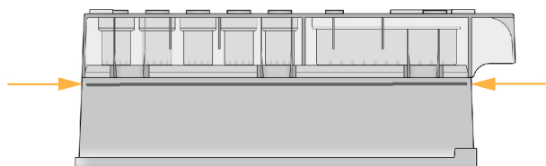
Figure 3 Maximum Water Line
